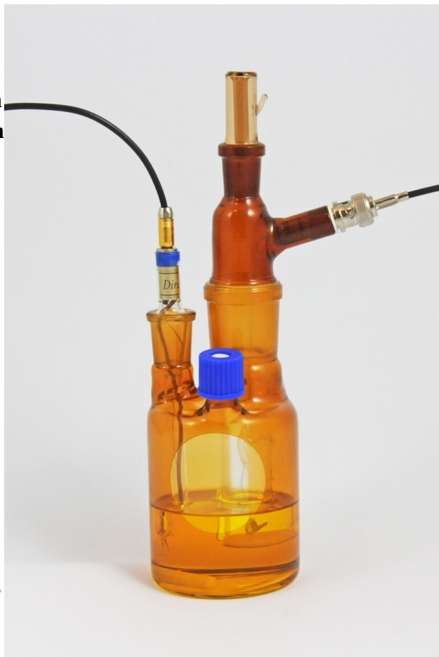
Figure 4: Titration vessel prepared for measurement
