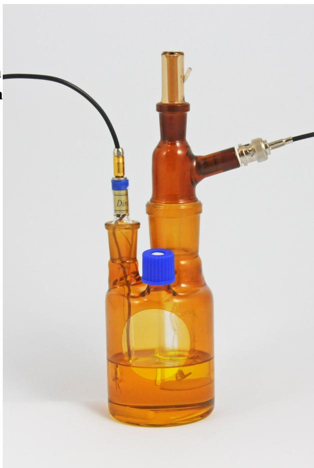
Figure 4: Titration vessel prepared for measurement
