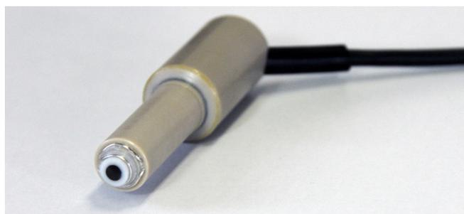
Figure 3: Electrode system of Aditest AP
