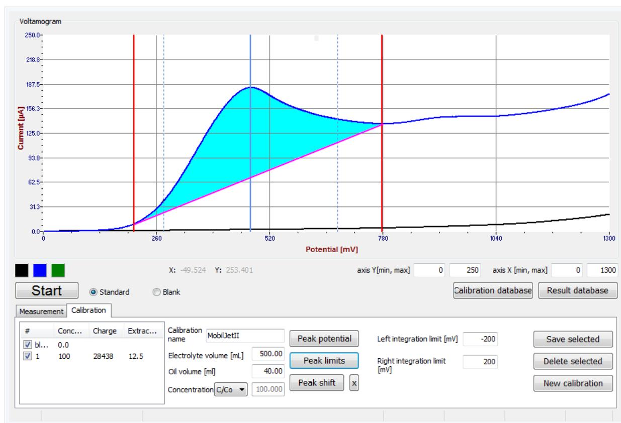
Figure 14: Correct determination of the peak area
