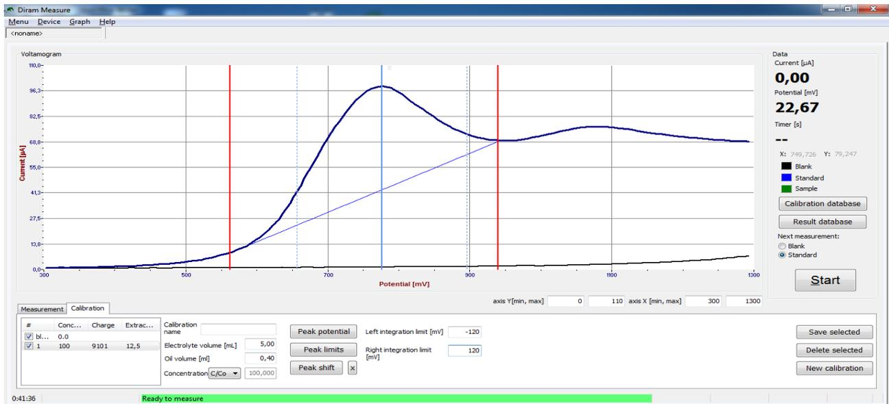
Figure 7: Peak potential - maximum (blue line), peak limits (red lines) and integration limits (blue dotted lines).
