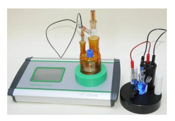
The neutralisation takes place in the closed cathodic compartment of the glass vessel which excludes possible interferences arising from the atmospheric carbon dioxide. The advantage of the coulometric method lies in minuscule solvent consumption and high accuracy of titrant metering, without the necessity to utilise standardised volumetric solution methods.
